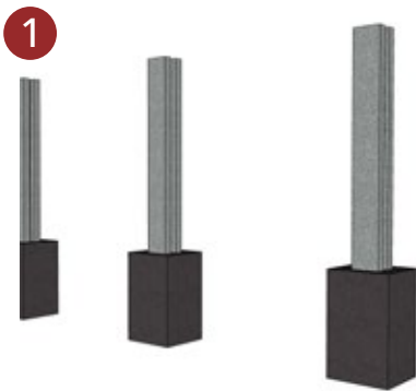
Erect H columns on footing
